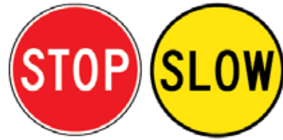
Figure 5: Hand-held stop sign used by a traffic controller. You must stop at a safe distance from the traffic controller and wait when facing a STOP bat. You may proceed with caution when faced with a SLOW bat.
