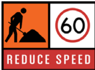
Figure 4: This multi-message sign warns motorists that there are roadworkers ahead on or adjacent to the road, and imposes a speed limit that applies until the next speed limit sign. You are required to reduce speed to, or below, the speed limit indicated.
