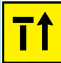
Figure 7: Left lane closed ahead. The T symbol indicates which lane is closed ahead and the arrow which lane or lanes remain open.
